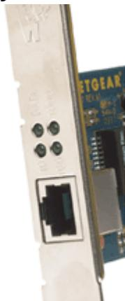
**Figure 3-1: Physical connection indicators on the front of the GA311 adapter**
