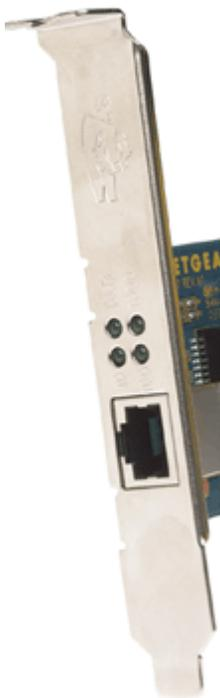
**Figure 4-2: Front of the GA311 Adapter**
